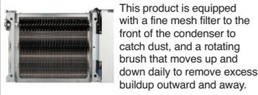
This product is equipped with a fine mesh filter to the front of the condenser to catch dust, and a rotating brush that moves up and down daily to remove excess buildup outward and away.
