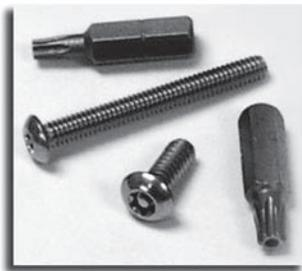
Special correctional model fasteners
